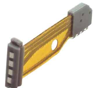
Custom Paliney® alloy, precision stamped and insert molded with Kapton® for corrosion resistant hearing aid connector
