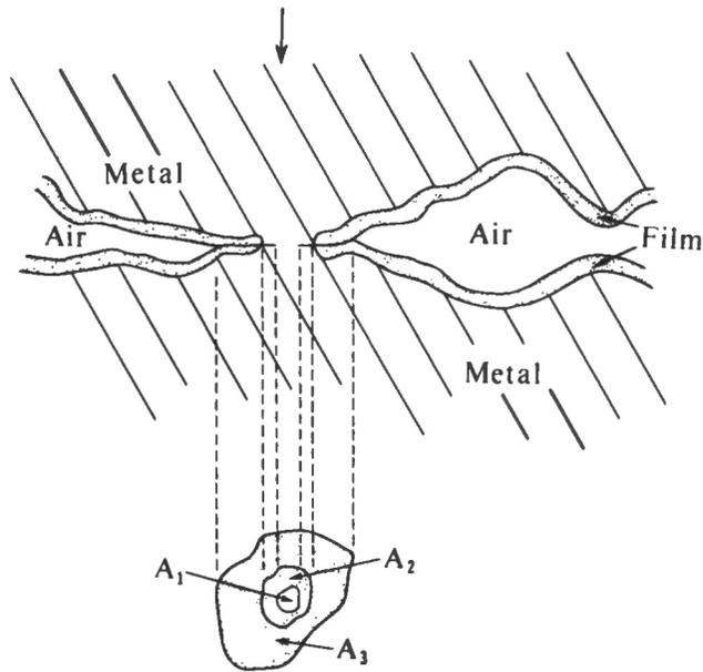
**Fig. 1-7. Condition after fritting.  $A_1$  is area of metallic bridge or microweld,  $A_2$  is where metals touch without weld; insulating films touch at  $A_3$ . All three areas help support the mechanical load  $P$ .**
