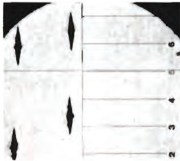
**Fig. 2-10. A portion of the view through the filar eyepiece of a microhardness tester.**
