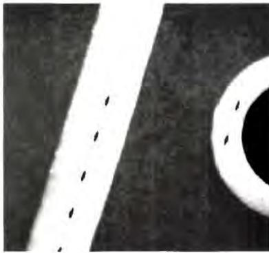
Fig. 2-8. Small parts with Knoop impressions. Magnification 67X.
