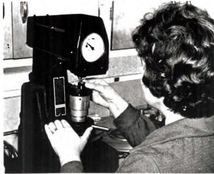
**Fig. 2-6. Rockwell superficial hardness machine being used to place "Brinell" hardness indentations in mounted specimen.**
