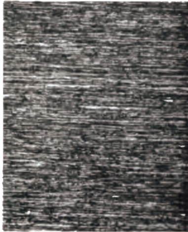
Fig. 2-24. Metallographic structure of Paliney ® 7 in the stress relieved condition. Note the similarity to work hardened structure, as shown in Fig. 2-21. Magnification 532X.
