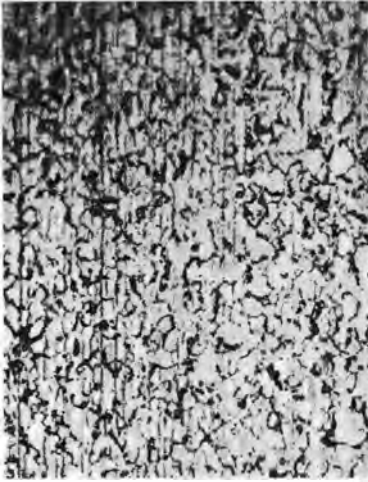
(a) Metallographic structure of Paliney® 7 in the Ductile HT (partially age hardened) condition. Magnification 532X.
