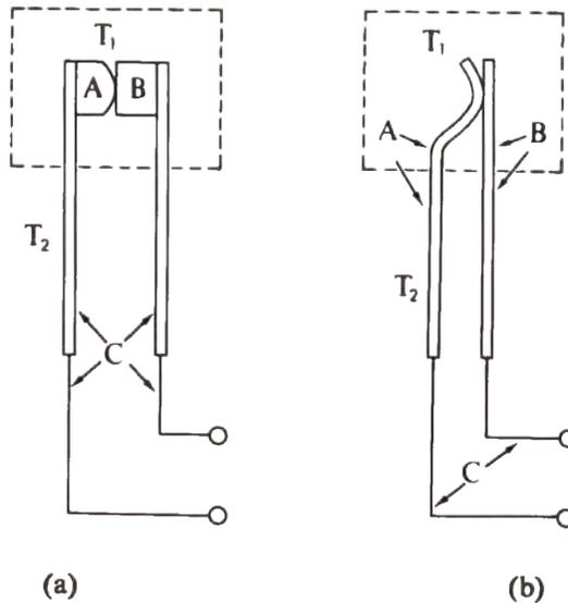
Fig. 2-40. (a) A circuit that will not produce a thermal emf.
