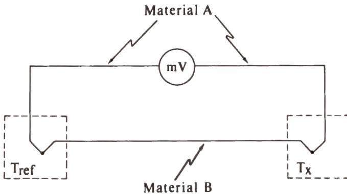
Fig. 2-39. A classical thermocouple circuit.
