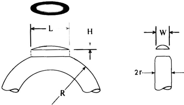
Fig. 4-4. Wear or erosion volume of formed wire operated against a flat surface.
