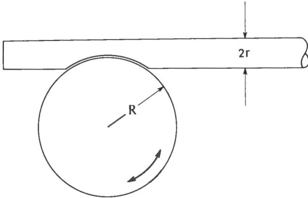
(a) Worn wire contacting a rotating ring.
