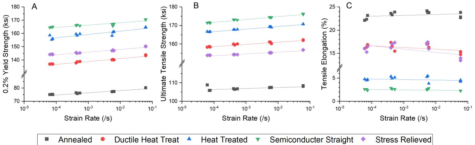
**Figure 2:** Comparisons of A) yield strength, B) ultimate tensile strength, and C) tensile elongation vs strain rate for all five tempers of Paliney® 7
