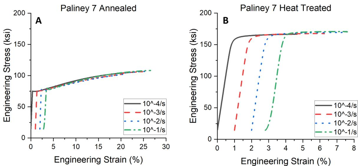
**Figure 1:** Stress-strain curve comparisons of Paliney® 7 at different strain rates in the A) annealed and B) heat treated conditions. Curves are offset by 1% strain for clarity.
