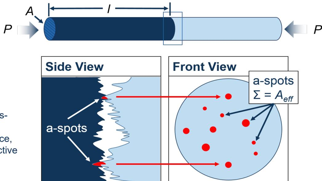
Figure 1: Schematics including contact dimensions discussed in the text (top) and example of a-spot formation leading to constriction resistance in metal-to-metal contact (bottom)
