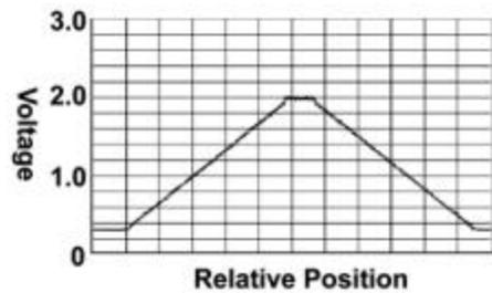
**Figure 12.** Voltage output for the new noble metal based conductive ink after a simulated 100,000 mile laboratory test. Contact material was Paliney<sup>®</sup> 6, bifurcated button with a normal force of 8.5 grams per finger.
