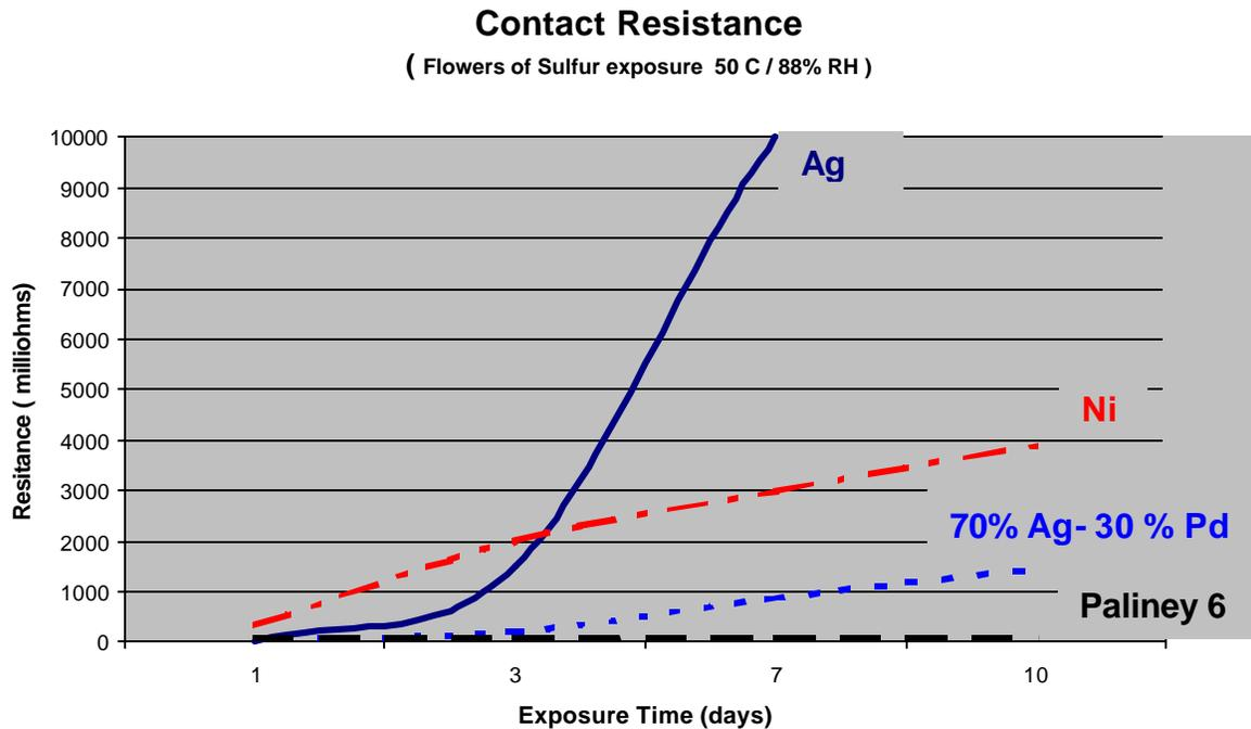
**Figure 14.** Static contact resistance measurements for typical sliding contact materials taken as function of exposure to a Flowers of Sulfur environment held at 50 C and 88% relative humidity. The sulfur rich environment is used for ranking purposes only and not meant to simulate reaction kinetics found in commercial gasolines.
