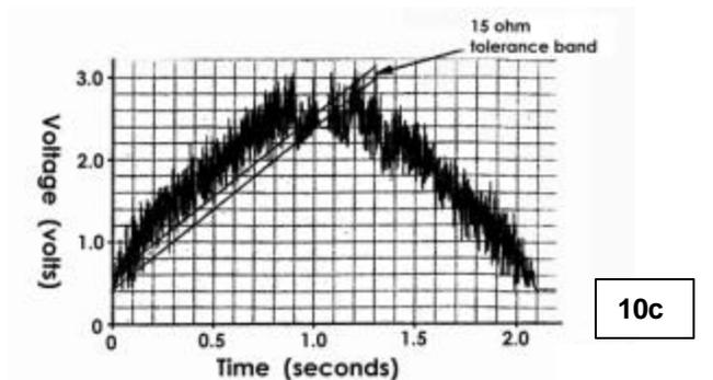
**Figure 10.** Examples of Ag rich layer that was adhesively transferred from the ink to the contact surface. a) surface SEM view, b) X-ray spectra of transferred layer showing sulfide tarnish, c) noise spectra from sulfide tarnished layer.
