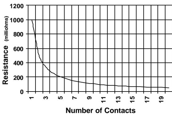
**Figure 16.** Theoretical calculation showing the reduction in contact resistance achieved by using multiple points of contact. The calculation assumes an initial uniform film resistance of 1000 mohms per individual finger.
