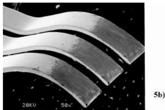
Figure 5) Minimal contact wear found after 1,125,000 cycles at 12 grams normal load using the segmented track and Paliney<sup>®</sup> 6 contacts
