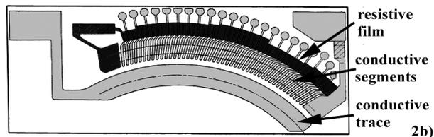
Figure 2) Schematic diagrams of the circuit traces
