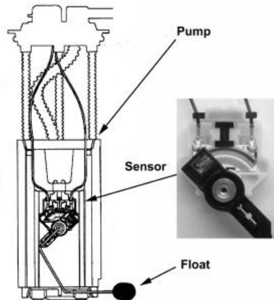
Figure 1) Schematic drawing of the fuel sender module showing a typical location of the fuel level sensor with an enlarged photograph of the sensor assembly
