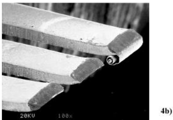
Figure 4) Severe contact wear after 600,000 cycles at 10 grams using the segmented track with C770 contacts
