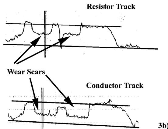
Figure 3) Wear characteristics of the original design, fuel level sensor after 300,000 rotations with a 15 gram load.
