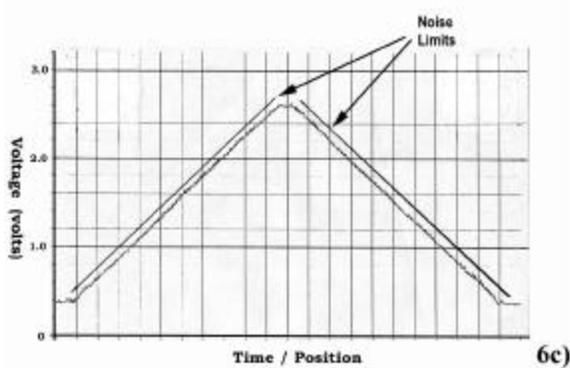
Figure 6) Voltage versus time plots for all three designs showing differences in noise levels
