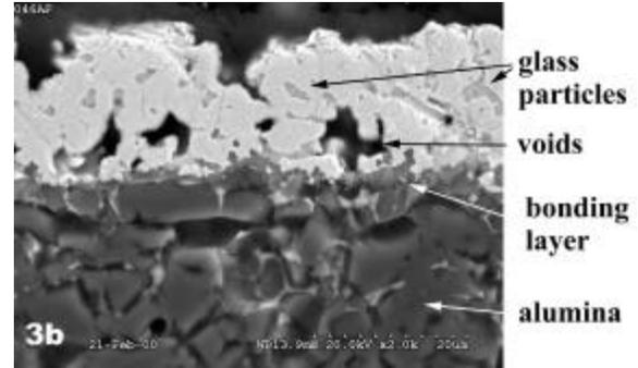
**Figure 3.** SEM photomicrographs of the surface (3a, 1000x) and cross sectional (3b, 2000x) views of the as fired coarse frit ink.
