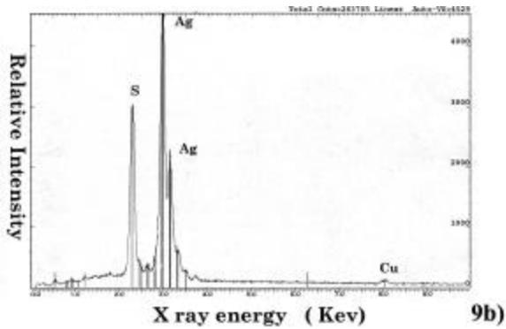
As seen in figure 8, the contact mated to the fine frit ink also showed evidence of abrasive wear, but at a much lower and more consistent level. As seen in figure 9, however, the contact mated to the mechanically smoothed surface shows evidence of adhesive transfer. The x-ray spectrum shows the transferred layer is silver rich with a significant sulfur peak.
