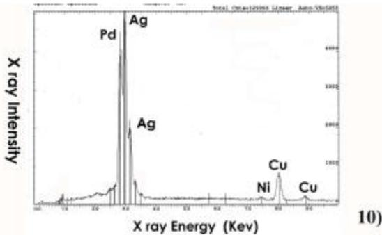
**Figure 10** X-ray spectra from a non-wear area of the sliding contact after 5 million cycles.
