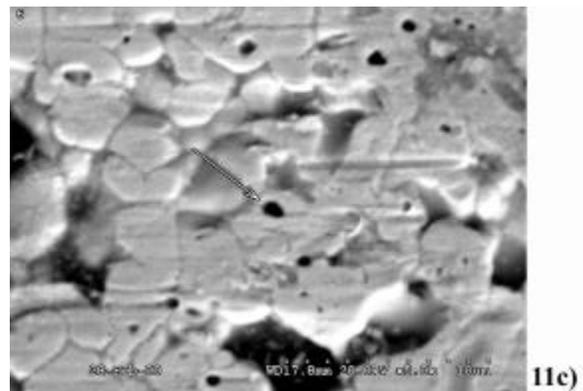
**Figure 11.** SEM photomicrographs of the two as fired ink surfaces after different levels of cyclic wear.
