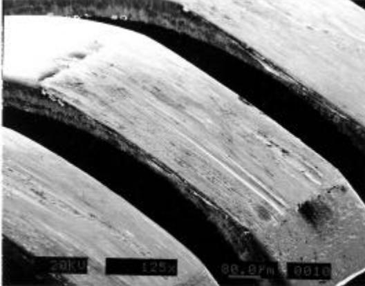
**Figure 7c.** SEM photomicrograph of contact wear after 250,000 cycles riding on the as fired, coarse frit glass.
