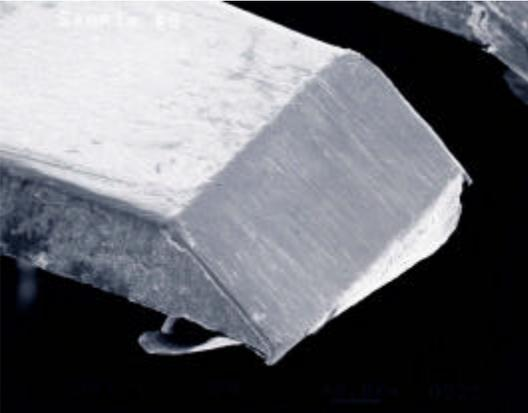
**Figure 7b.** Surface SEM photomicrograph of a sliding contact from a second sample after only 4.0 million cycles mated against the as fired, coarse frit ink.
