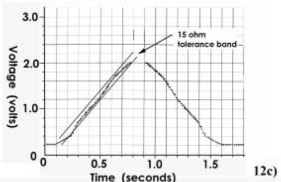
**Figure 12.** Electrical output of fuel level sensors from each of the three inks
