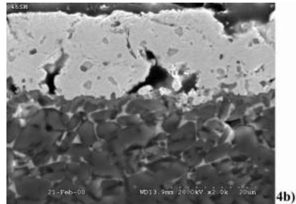
**Figure 4.** SEM photomicrographs of the surface (4a, 1000x) and cross sectional (4b, 2000x) views of the mechanically polished ink.
