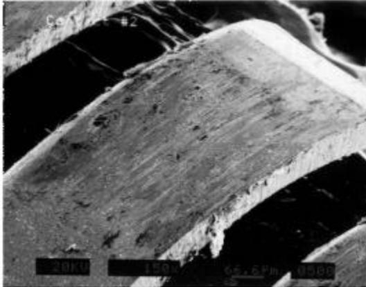
**Figure 7a.** Surface SEM photomicrograph of a sliding contact after 5.3 million cycles mated against the as fired, coarse frit ink.
