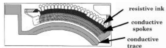
**Figure 2.** Schematic diagram of the circuit traces.
