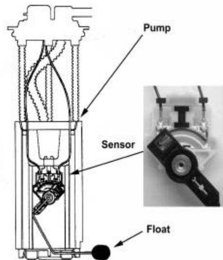
**Figure 1.** Schematic diagram illustrating the fuel sender module and position of the level sensor.
